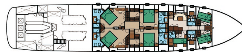
Lower deck Standard version 4 cabins + crew cabin
