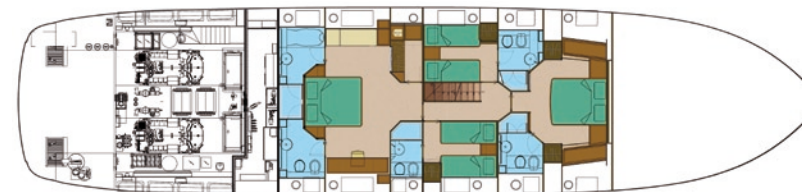
Lower deck Standard version 4 cabins + crew cabin
