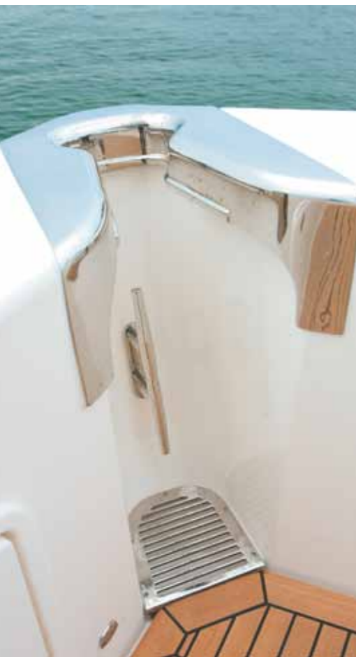
The triple IPS600s (above right) are big and impressive, and give the Riviera 53 a high-bow attitude underway (top), but cut 1000kg of the weight from equivalent engines in shaftdrive mode. Crew will be secure berthing the 53 with open-ended hawsepipes and oversize cleats in the transom corners (above).
