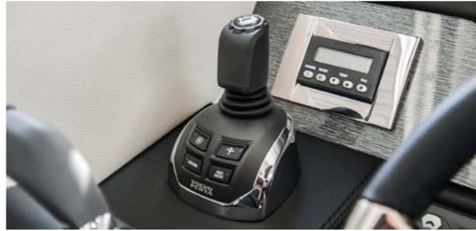
Volvo Penta's innovative Dynamic Positioning System (DPS) is an excellent option for simple yet effective station-holding while preparing lines and fenders or while waiting off a fuel jetty.
